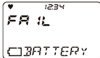
Battery voltage abnormality
