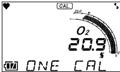
(14) Connect the gas sampling bag in which the O<sub>2</sub> calibration gas was collected to the gas inlet to supply the gas to the gas detector. Wait for the concentration display value to be stabilized.
