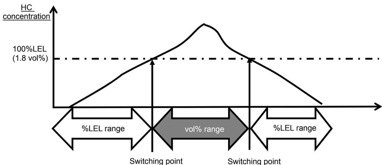
\* HC: The acronym of HydroCarbons. Because combustible gas concentration is displayed in isobutane conversion in this detector, the range switching point is LEL 1.8 vol% of isobutane.
