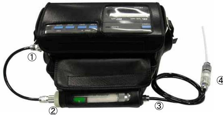
For gas sampling, 3 kinds tip formation are available and change it according to the measuring environment.
