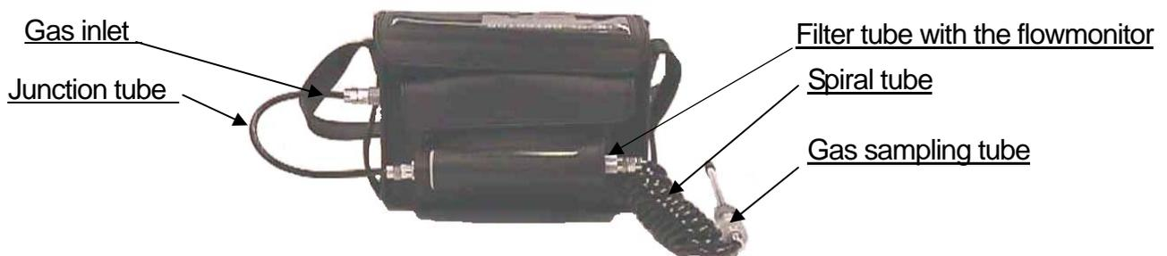
As there are two types of head tubes for the instrument, use it according to the each environment.
