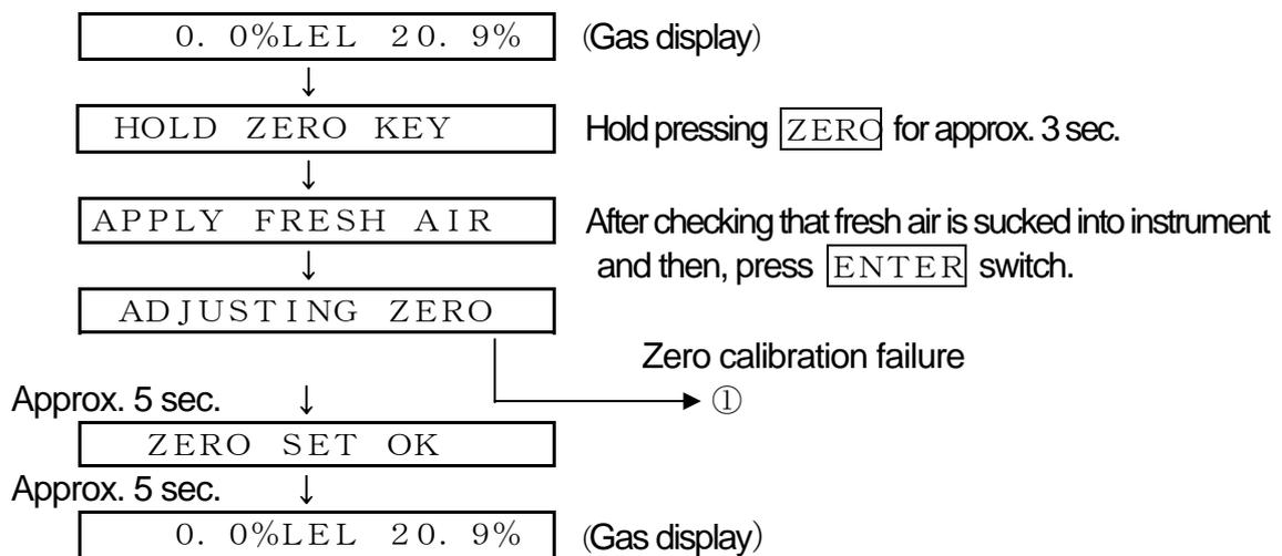
① Display, performance at zero calibration failure (See 3.)
