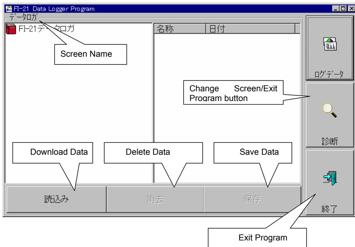
To communicate the data, connect the communication cable to the Model FI-21. Once PC's power is ON, it will judge automatically whether or not communication is possible. If it is possible, the PC will be ready to receive the data.
