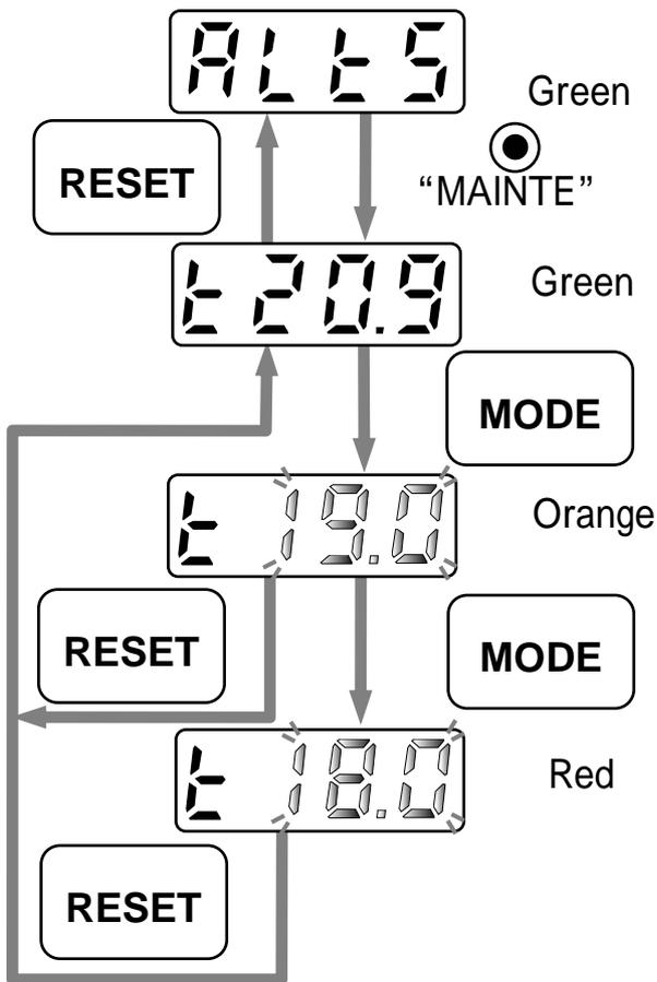
"t" which is located in the left side of the test rate will be indicated in Green.
