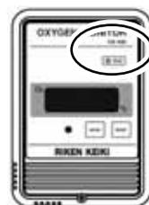
When OX concentration decreases again and becomes below 18.0% [standard], the alarm lamp (orange, red) will start to flash and the continuous buzzer sound will start beeping.
