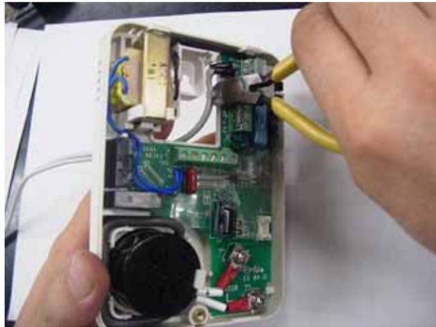
Let cable clamp through the upper part of the hole to pull out cable and fasten the cable clamp halfway.
