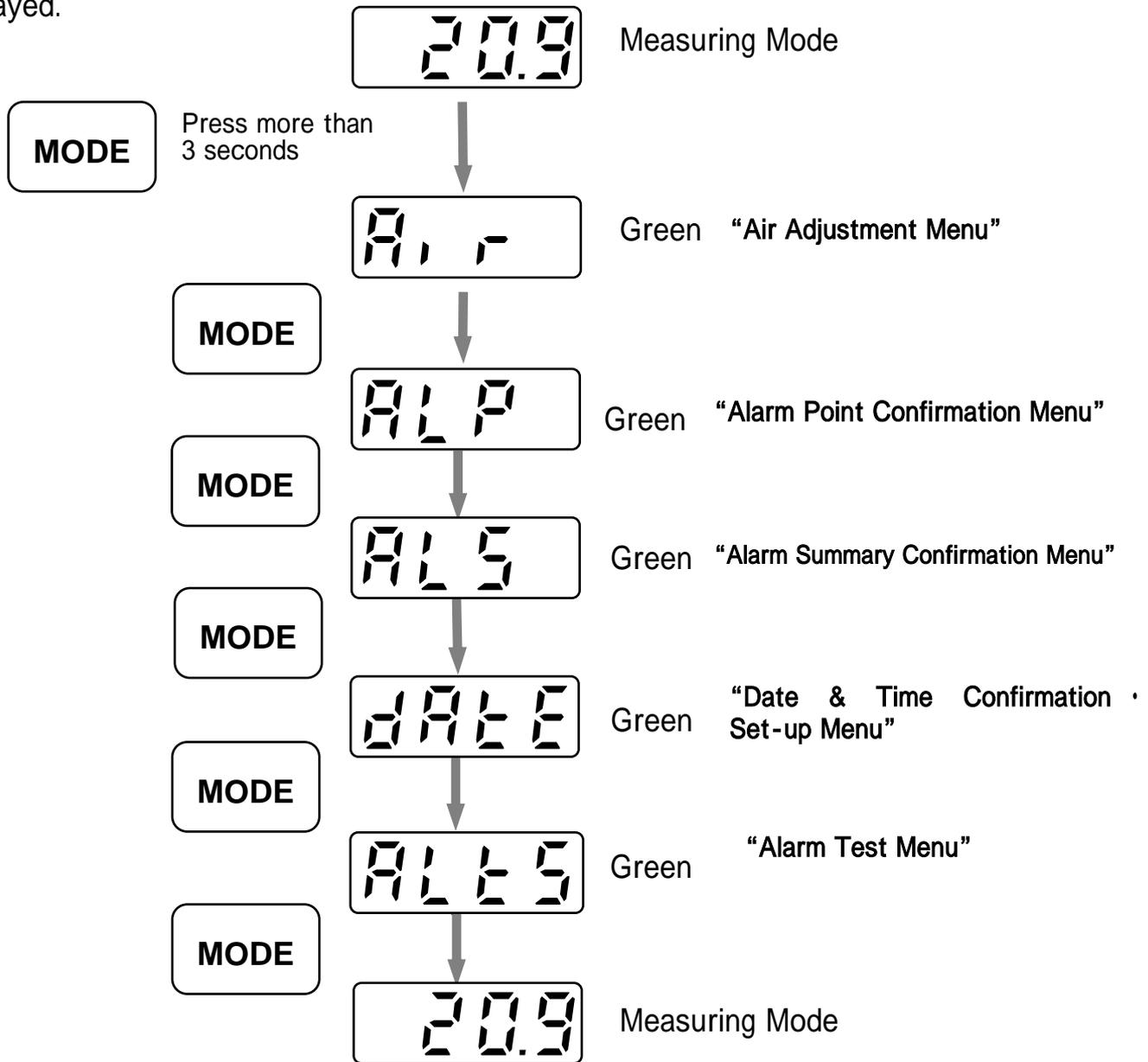
While the "User's Maintenance Mode" is displayed on instrument screen and if you don't operate more than 1 minute, notice of completion bell will ring and it will return to the "Measuring Mode".
