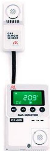
The **OX-600** is an indoor, standalone monitor that detects Oxygen (O<sub>2</sub>) with a range of 0-25 % volume with 0.1% increments. Its compact, lightweight low profile design is equipped with a unique tri-colour display, which changes colour as oxygen levels reach
